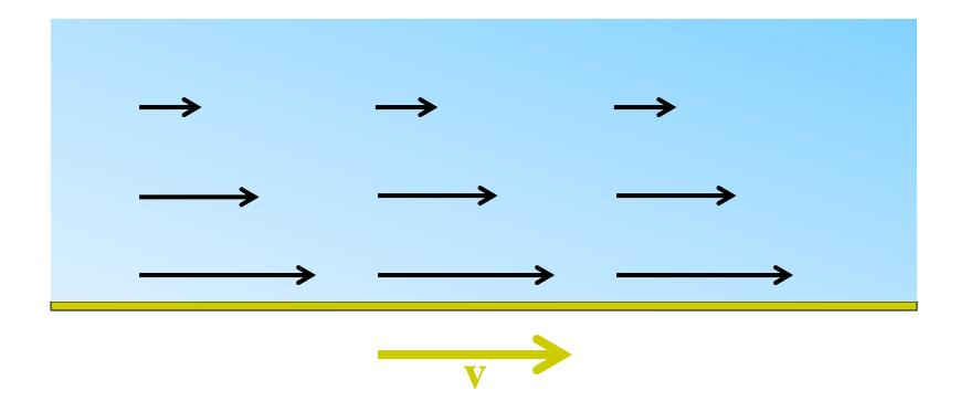
Viscosity = [(force/area)] per unit velocity gradient
