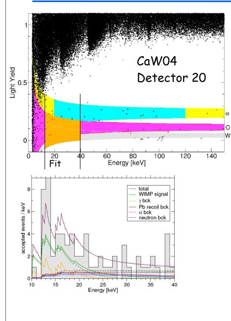
Detailed fit of recoil energy and scintillation distributions + multiplicity (neutrons)
