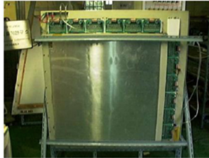
Fig. 2. 2 mm double gap RPC manufactured for the gamma ray transmission images.
