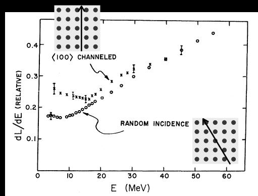
FIG. 11. Scintillation efficiency dL/dE as a function of incident-ion energy for <sup>16</sup>O ions on NaI(Tl), for both random incidence and for channeling along a  $\langle 100 \rangle$  axis.
