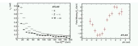
Figure 9: (left) Accuracy of the measurement of the azimuth of the  $\not\!\!E_T$  vector as a function of the true  $\not\!\!E_T$  for three different physics processes: semi-leptonic  $t\bar{t}$  events,  $Z \to \tau \tau$  and  $W \to ev$  events. (right)  $\not\!\!E_T^{\text{Fake}}$  as a function of the reconstructed  $\phi(\not\!\!E_T)$  in  $t\bar{t}$  events, simulated with extra material in  $\phi$ .
